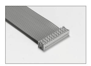
These ID transition connectors are mainly used for a permanent connection to the PCB. The pin portion of the circuits are on a 2.54mm spacing which fits the fully shrouded header mounting hole layout. Bodies and covers are supplied pre-assembled. Connectors are suitable for stranded conductors AWG 28.
