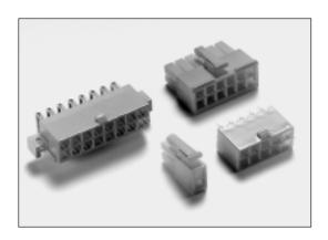
A new multi pin connector family for currents from 6 to 9 AMP per circuit (depending on circuit size). Terminals are fully isolated. Housings are positive locked and terminals have multiple point contact for lower insertion/withdrawal forces.
