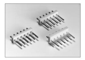
1.14mm square or round pins pre-inserted into polyester wafers that are a low cost means of interconnection. Mates with TLS series crimp or ID style connectors and TLS series PCB solder connectors. Besides the standard pin length of 19.05mm other pin lengths are available, up to a maximum pin length of 97.28mm.
