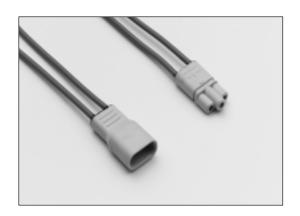
A choice of 2 and 3 way high reliability cable to cable power connectors with machine tooled crimp and solder-bucket terminals. Housings are fully polarised and include latching mechanisms for added strain relief. Incorporated in the housing design is an '0' ring seal which, when combined with back potting the connector achieves IP55 and 67 ratings.
