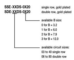
Selection 0 is PC/104 non-stackthrough (2 x 20/2 x 32 = stock item). Selection 3 is PC/104 stackthrough (2 x 20/2x 32 = stock item). Other circuit sizes are subject to (M.O.Q.).
