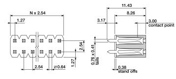
Recommended insertion depth = 5.97mm (max.) PCB Hole Size = Ø1.00mm
