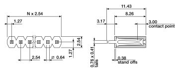
Recommended insertion depth = 5.97mm (max.) PCB Hole Size = Ø1.00mm
