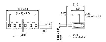
Recommended insertion depth = 2.67mm (max.) PCB Hole Size =  $\emptyset 1.00mm$
