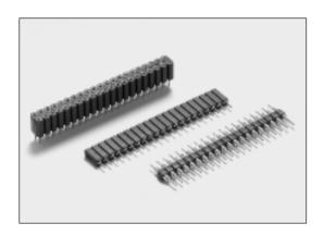
A range of professional socket and header strips with machine tooled contacts. Socket contacts are of a two part construction. An outer shell with an inner four fingered spring contact. Sockets accept round pins from Ø0.65mm to Ø0.85mm and square pins from 0.62mm to 0.65mm.
