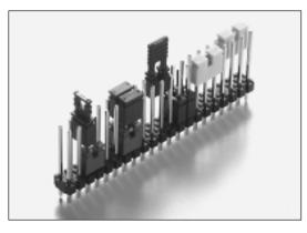
Programming shunts. All models have a double sided contact design. Open and closed models have fingernail grip design for easy removal by hand. The open models 5100/5126 are supplied on strips of 20 pcs for easy installation
