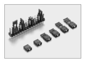
A newly designed family of shunts with a unique all around finger grip for easy removal from male headers. These shunts are designed to be placed side by side or back to back and have a special design which protects them against being mis-placed (male pin cannot be placed in between the two contacts). Contact point is 4.15mm from the bottom.
