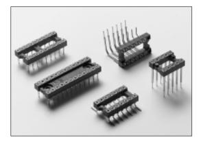
This complete range of professional DIL sockets have machine tooled contacts. The contacts are of a two part construction, an outer shell fitted with an inner four fingered spring contact. For all sockets the combination of a tin plated shell/pin and a gold plated clip is standard. Tin plated and thicker plated clips are available against M.O.Q. Please contact sales office for more information.
