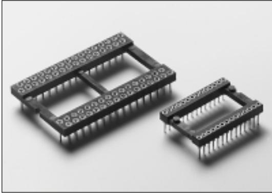
Some special type IC sockets with machine tooled contacts. All are of a two part construction, an outer shell filled with an inner four-fingered spring contact.
