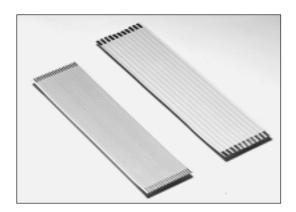
These compact, lightweight and thin flat cable jumpers are ideal for designing miniature equipment and high density mounting in combination with available FFC connectors. For greater flexibility, conductor thickness can be reduced to 0.05 or 0.035mm.
