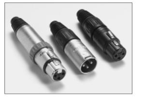
These professional Neutrik connectors are accepted as standard, worldwide. They have rugged die cast shell, compact design, time saving assembly (4 parts only), no screws and are equipped with the unique chunk type strain relief. Back sleeve is coloured black as standard. For identification 10 different coloured sleeves are available. Right-angle models have a 7 x 45° index possibility.
