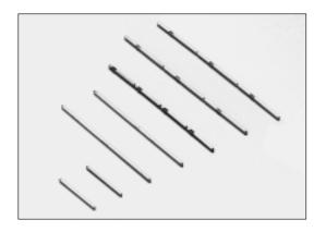
Square pins for wire wrapping, connector or test point applications. The square plain pins are available as loose pieces. Recommended hole size is  $\emptyset 0.74$ mm  $\pm 0.05$ mm. The square star pins are supplied in joined strips, in packs of 1000 pieces. Recommended hole size is  $\emptyset 0.80$ mm  $\pm 0.05$ mm. Contact sales office for hand held tool with adjustable spring impact head.
