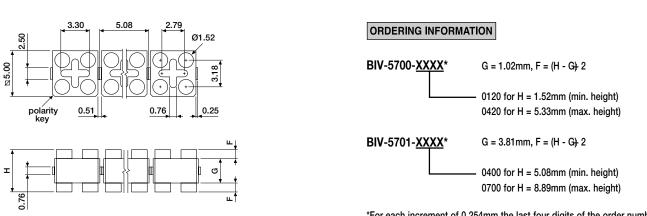
\*For each increment of 0.254mm the last four digits of the order number must be increased by 20.
