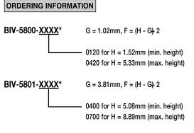
\*For each increment of 0.254mm the last four digits of the order number must be increased by 20. Contact sales office for LED's holders assembled with LED's and see
