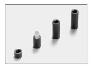
Self-retaining design makes assemblies suitable for automatic insertion. Unique design of lead exit holes allows self retention and draining of cleaning solvents. Standard heights from 3.05mm to 22.86mm with various increments.
