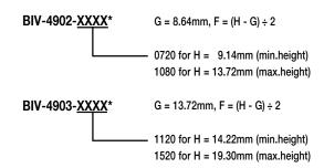
\*For each increment of 0.508mm the last four digits of the order number must be increased by 40.
