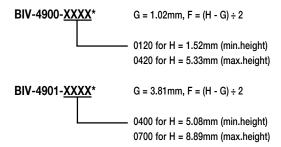
\*For each increment of 0.254mm the last four digits of the order number must be increased by 20.
