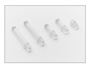
Light pipes are ideal for applications where an automatically placed SM LED needs to have it's output redirected to a front panel or enclosure. Light pipes are produced from clear polycarbonate for maximum light transmission. Light pipes will also protect circuits from accidental damage from ESD by isolating the PCB from potential contact.
