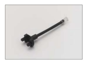
These revolutionary proprietry flexible light pipes allow the ultimate in design flexibility. SMD or through hole LED's can be positioned anywhere on the PCB and still provide a bright high contrast front panel indicator. Two piece design, indicator and light pipe press fit together assuring tight retention and shock resistance.
