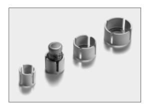
These mounts protect components from shock and vibration with resilient shock absorbing, vibration damping mounting, from high temperatures during soldering by spacing with a heat buffering fixture and keeping lead origins away from all solder. Prevent short circuiting, bridging and moisture built by elevating insulating components.
