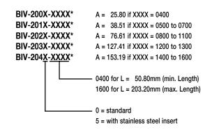
\*For each increment of 12.70mm the last four digits of the order number must be increased by 100.
