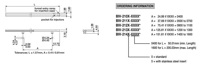
\*For each increment of 12.70mm the last four digits of the order number must be increased by 100.
