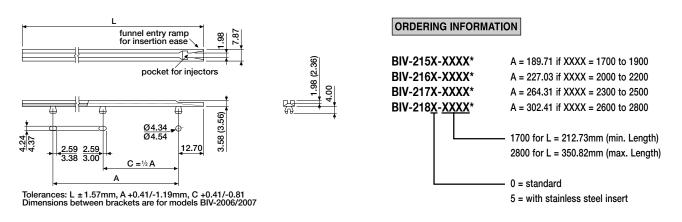
\*For each increment of 12.70mm the last four digits of the order number must be increased by 100.
