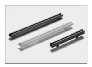
These guides have a 5.08mm slot depth providing maximum board retention for wide boards and high vibration and shock applications. The guides are double ended, with panel entry, so that they may be used in various length combinations to obtain virtually any overall length desired. All card guides can be supplied with a stainless steel channel insert for EMI/RFI protection.
