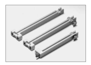
Card guides for vertical mounting with integrally moulded metal threaded M3 inserts and with a unique push-button lock option. Anti-vibration features in the card slots prevent sideway movement of the PCB. All models have, at both sides, guide grooves and have a v-shape PCB entry for easy loading.
