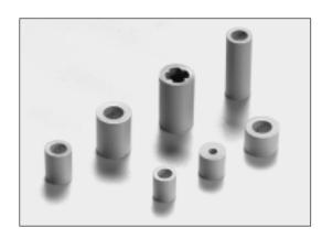
Seventeen basic I.D./O.D. combinations for the standard spacers and nine for the self-retaining models. Heights ranging from 0.76 to 31.75mm in 0.127mm increments and from 1.00 to 26.00mm in 1.00mm increments are available. Models 1250/51/52 and 1260 have a unique bi-material design.
