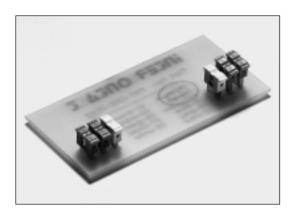
This single circuit IDC contact accepts flexible hook-up wire from AWG 26 - 22 (0.14 - 0.34mm²). The contact can be used for a maximum of two wires. Wires can be placed and removed without using tools, by simple pressing or lifting of the plastic upper part.
