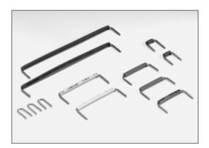
Jumper wires can be used for making interconnections on PCB's. 14 different lengths are available. Jumper wires are made of solid AWG 22 PVC insulated copper wire. Any special wire jumper, insulated, uninsulated, or insulated with Teflon®, Kynar®, etc., can be produced on request.
